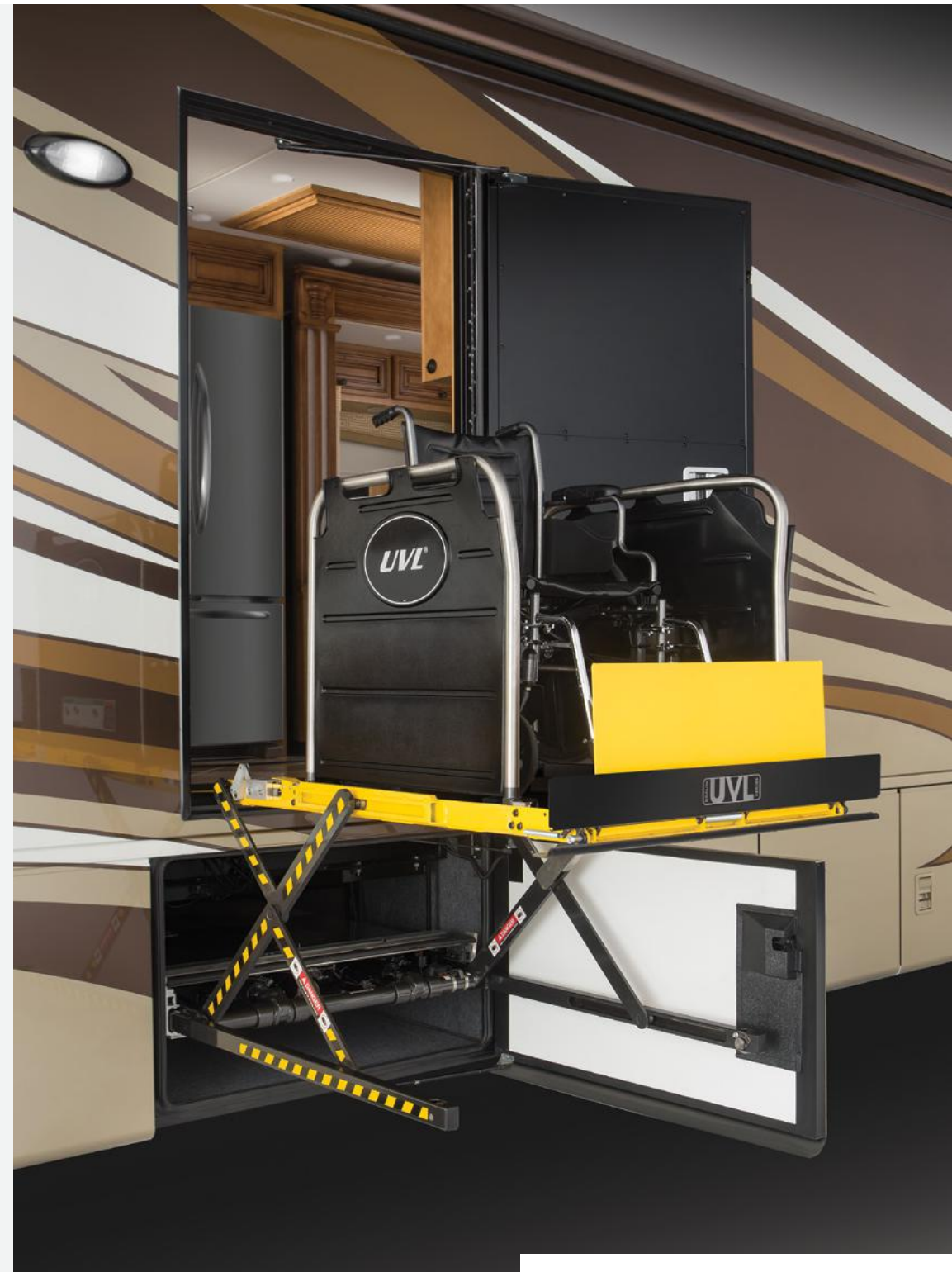
Remote-Control Lift with Access Door
